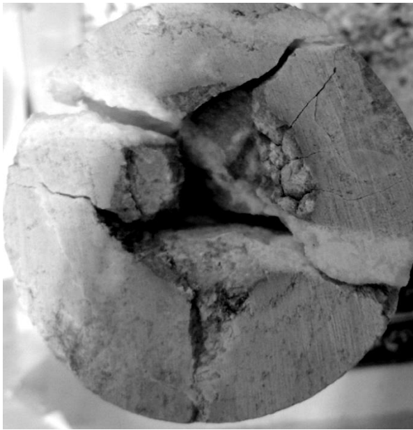
Figure 11: Experimental result of Limestone under plasma torch test. Damages and fractures are macroscopic and visible.
