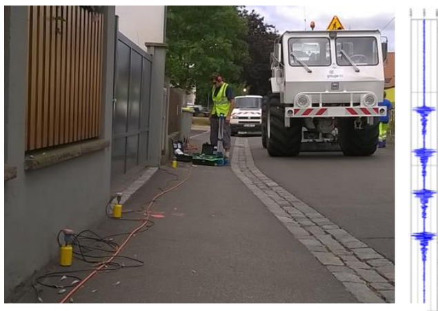
Figure 4: The picture on the left side shows the single vibroseismic truck used inside the city, the geophones layout along the road and the vibration monitoring made at each vibrated point. The seismogram on the right side was the output of the vibration monitoring (PGV in mm/s)
