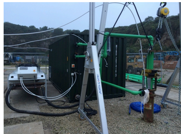
Figure 4 400kW Thermal Response Test rig with "air blaster" – external and internal viewpoints
