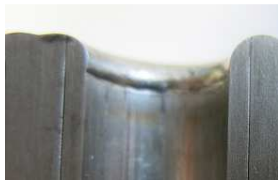
Figure 3: View of a welding model showing a lack of fusion
