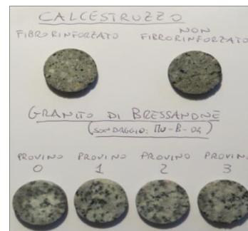
Figure 5: Rock and shotcrete samples for laboratory thermal conductivity and diffusivity tests.
