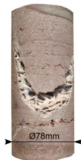
Figure 1: Photo of fractured Buntsandstein core from exploration well EPS1 at 1374 m depth. The rock contains a large fracture of roughly 1 cm in width, with precipitated barite crystals. Taken from Griffiths et al. (2016).
