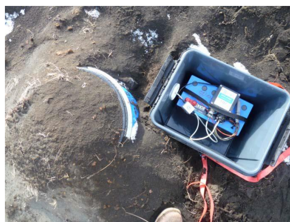
Figure 3: Sketch and example of an IMAGE on-land station. The sensor is placed on bedrock about 70 cm deep in the soil protected by a plastic barrel. The Cube data logger and power supply are in plastic box next to the barrel.
