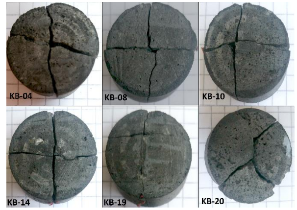
Figure 2: Photographs of the samples. The vertical fracture in all of the photos is the first fracture generation, and the horizontal fracture is the second generation. The samples are 26 mm in diameter.
