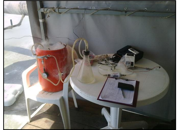
Figure 5: In situ measurements of gas/steam ratio.
