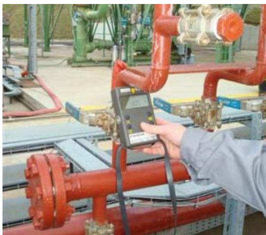
Figure 1: Dose rate measurement performed with the radimeter.
