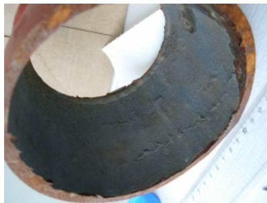
Figure 7: Pipe removed from the reinjection line and covered with black deposits
