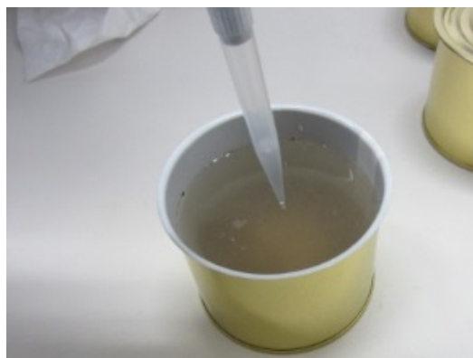
Figure 9: Fluid sampling from tinplate capsules as a function of the experimental duration (Picture: BWG).
