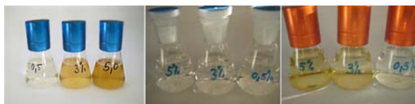
Figure 4: Artificial Soultz brine mixed with different concentrations of inhibitors. No precipitation of Ca-Phosphate was observed. Inhibitor Blue (left), Inhibitor Green (middle) and Inhibitor Red (right) (Picture: BWG).
