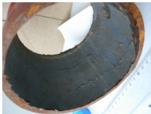
Figure 2: Barite scaling cover the inner surface of a pipe of the surface installations. The deposit has a thickness of 0.5 to 0.7 mm (Picture: GEIE).
