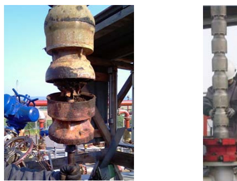
Figure 14: Status of the hydraulic part of the LSP pump after the pull operation of April 2011 (left) and picture of the new hydraulic LSP pump (right).
