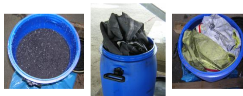
Figure 2: Typical radioactive residues from a geothermal power plant: scales (left), filter (middle) and combustible byproducts (right)
