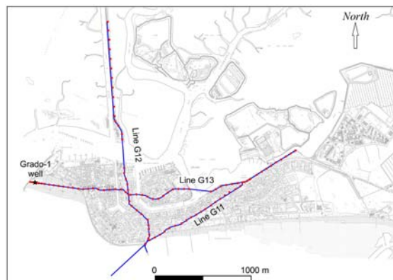
Figure 1: Location map of the surface seismic reflection (blue lines) and of the gravity stations (red points) along the seismic lines. The Grado-1 well (black star) is also indicated.
