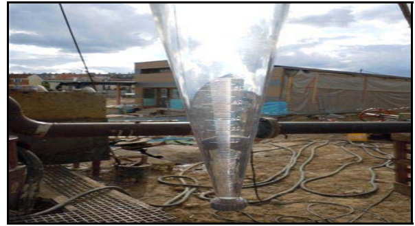
Figure 9: Checking of the solid content during the pumping test using Ihmoff cone
