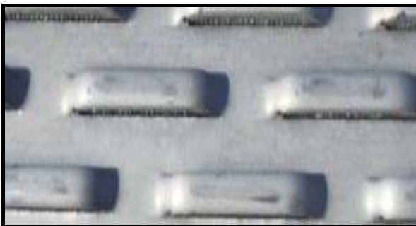
Figure 11: Detail of the screens (glass balls 0,3 to 1,4 mm) can be seen in the slit
