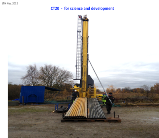
Figure 6: The National infrastructure for deep coring and sampling. Atlas Copco CT20.
