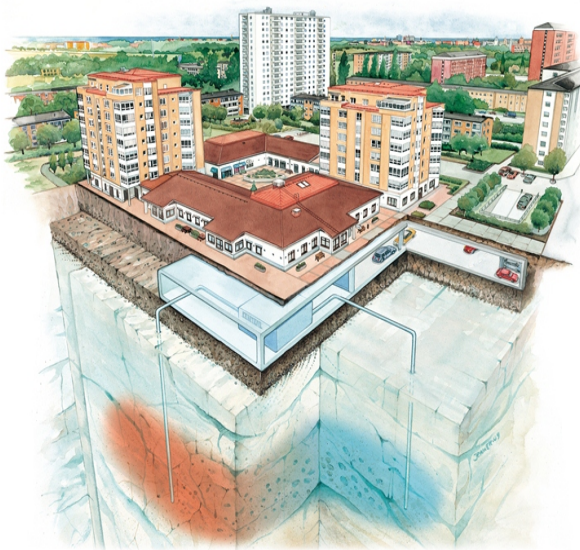
Figure 2: The principal of ATES, an open loop concept, where heat and cold are seasonally stored in an aquifer
