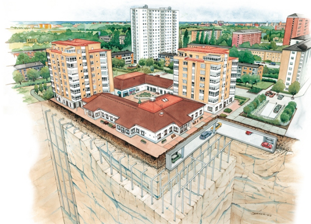
Figure 5: The principle of BTES, a closed loop concept, where heat and cold are seasonally stored in a solid rock mass through a large number of densely spaced boreholes.
