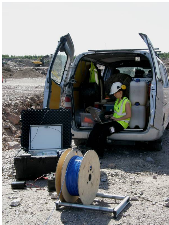
Figure 2: Distributed temperature system (DTS) measurements with fibre optic cable. Photo by I. Martinkauppi
