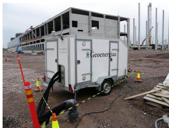
Figure 3: The first Finnish thermal response test unit (TRT) in operation at an industrial building area. Photo I. Martinkauppi
