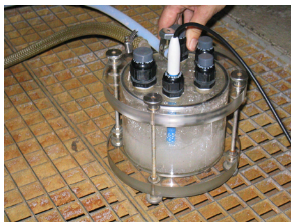
Figure 2: Thermal water sampling equipment Degassing processes after release of pressure are responsible for bubble formation in the flow cell.
