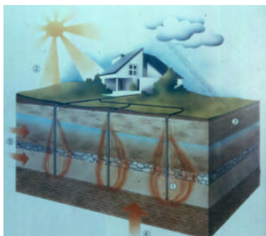
Figure 2: Principle of Ground Source Heat Pump System
