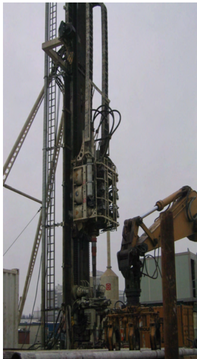
Figure 1: Derrick of the wells UHA GT 1 and GT 1A, the height of the derrick is only 19 [m].
