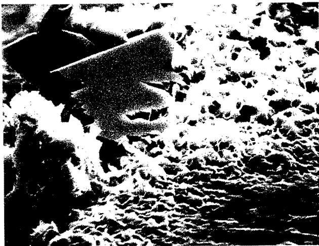
Figure 25. Nearly pure silicate minerals (EDAX scan shows only Si) adjacent to honeycomb clays (Fe, Mg, Al rich) overgrowths. Both features greatly reduce permeability. Sample from well M-3, at 2203 m depth. Field of view across the SEM photograph is 0.05 mm.
