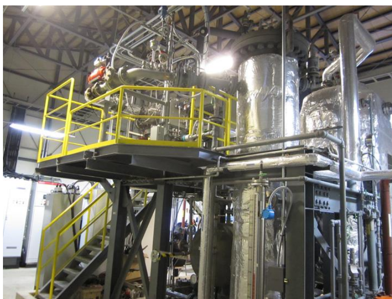
Figure 6: Kalina power generation system using hot spring fluid at Matsunoyama
