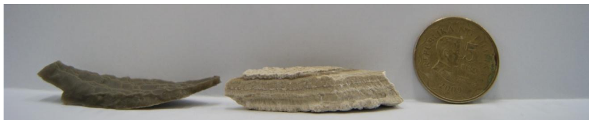
Figure 6. Scale samples collected in June 2013 (leftmost) and February 2013 (middle)
