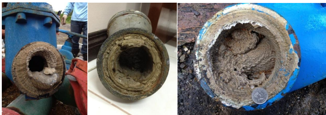
Figure 3. Massive depositions at joints, elbows and valves
