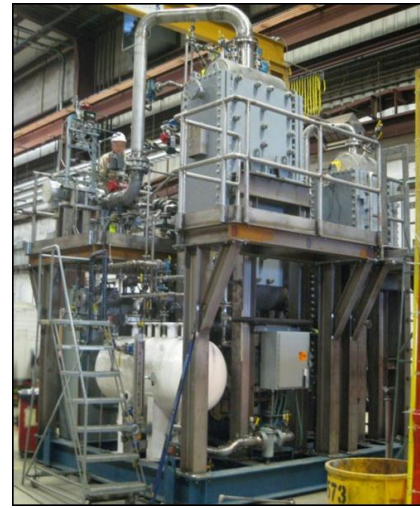
Fig.2 Kalina power generation system
