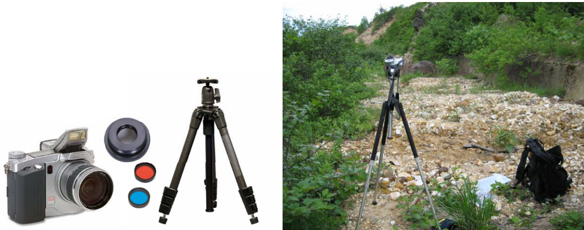
Fig. 4 CCD boasts 5.2 million pixels camera, filter, filter holder, and ball head tripod.
