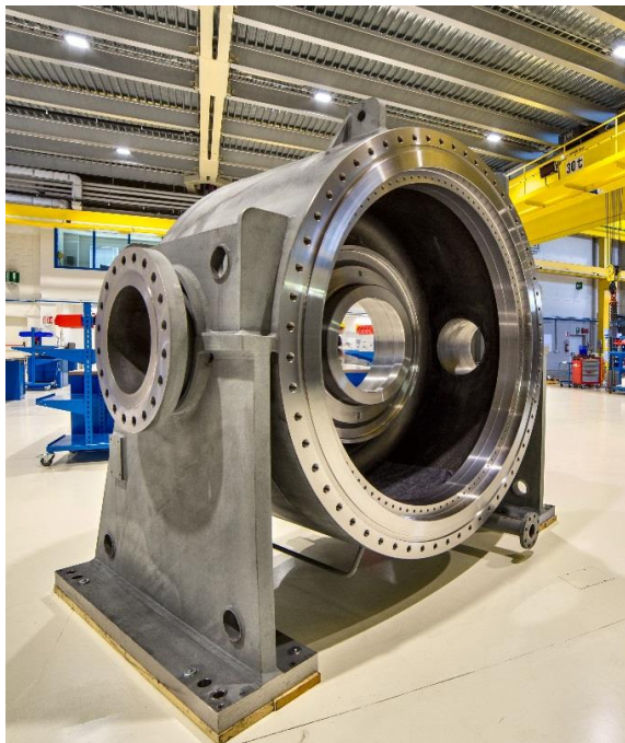
Figure 6 – The turbine for Velika Ciglana (15MW) is the first one with the new frame for application up to 20MW
