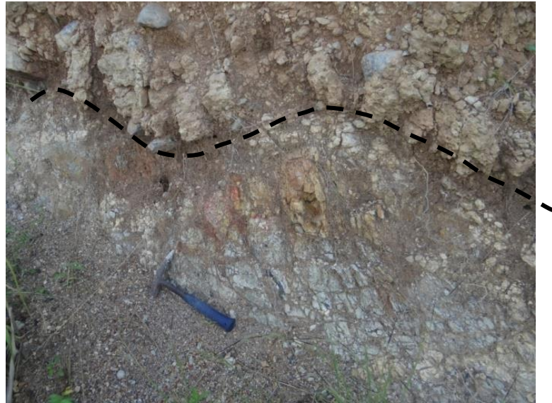
Figure 6: Hydrothermally altered mylonitic rocks (below dotted line) overlaid by bentonite (above dotted line) that cemented the cobbles and gravels. The travertine-deposits occur in cracks of the altered mylonites.
