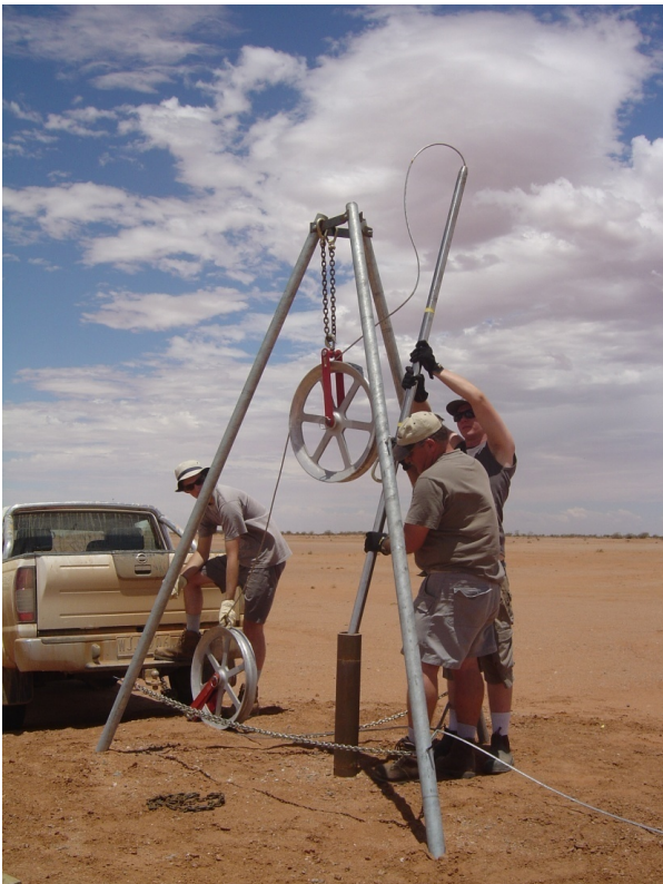
Figure 3: 15Hz Sensor being deployed into the Paralana-1b borehole. Station name = B05
