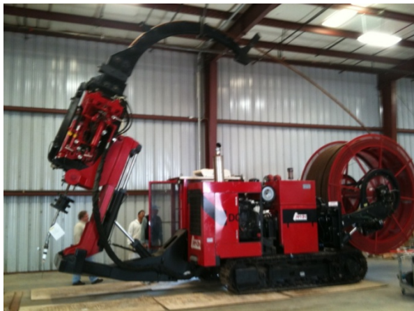
Figure 8: Coiled tubing unit for field testing of hydrothermal spallation well enhancement.
