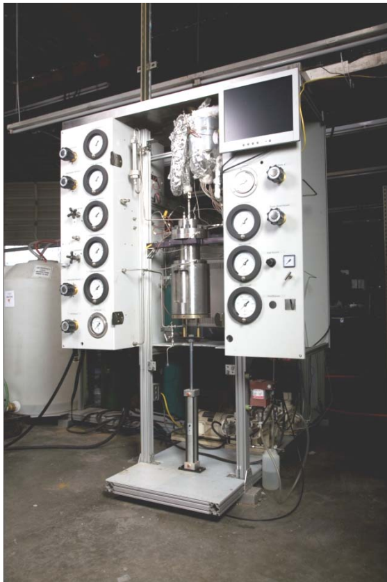
Figure 4: Hydrothermal spallation deep well test rig This system which uses superheated steam to spall the rock was used to create single axial slots of the desired depth in holes and investigate their interactions with induced fractures.
