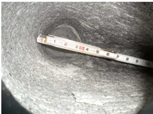
Figure 5: Axial slots cut into 10 cm open hole section of Sierra White Granite using a full scale tool
