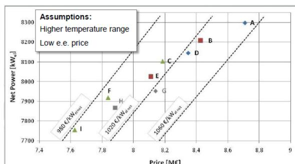
The table shows price/power ratios for different possible configurations of an air-cooled ORC unit (installed, BoP excluded) for the same Project.
