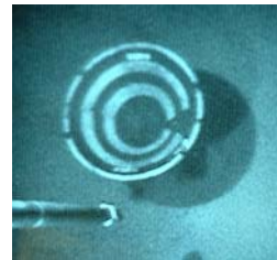
FIG. 18 – IODP RE-ENTRY CONE ON FLUID HAMMER 260 & CWD INSERTED CASING
