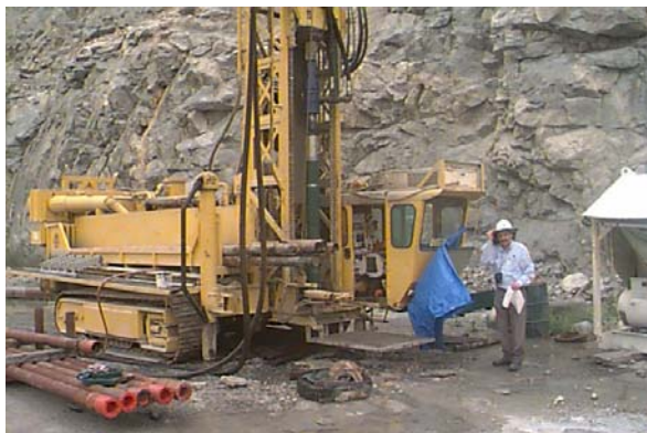
FIG. 12 – QUARRY TEST 8 1/2" PROTOTYPES
