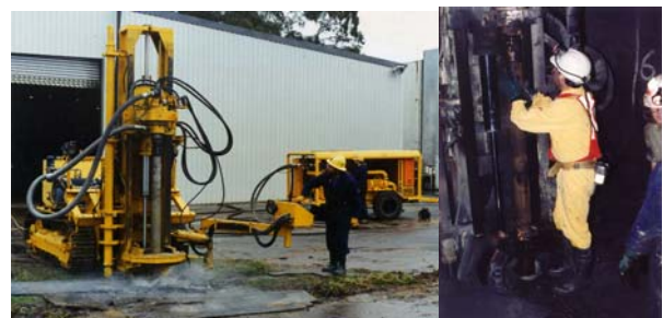
FIG. 4 – WATER HAMMER PROTOTYPE TESTING WITH GRANITE & UNDERGROUND
