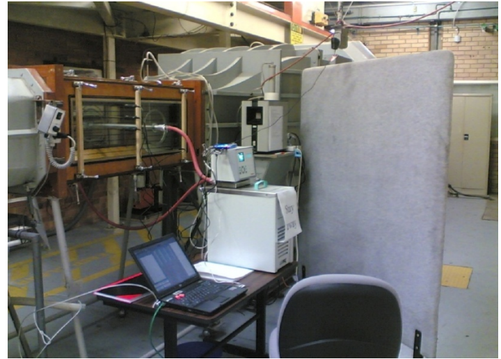
Figure 4: The low speed wind tunnel test facility; the hot water circulator and data acquisition system (sitting on the desk).
