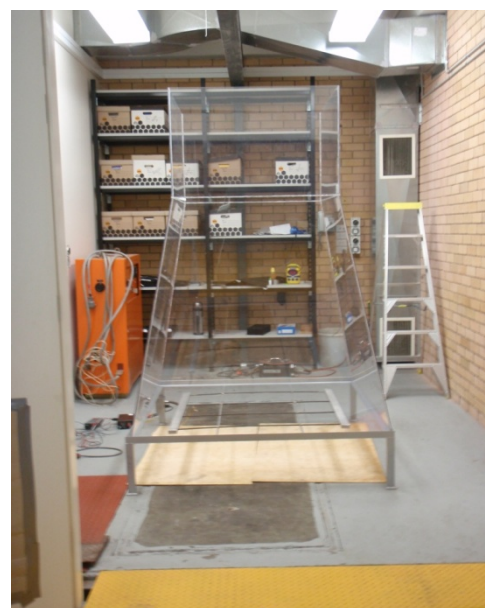
Figure 1: The QGECE lab scale model for a NDDCT.
