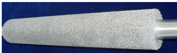
Figure 3: The metal foam-wrapped tube used in QGECE labs to conduct experiments on air-cooled condensers.
