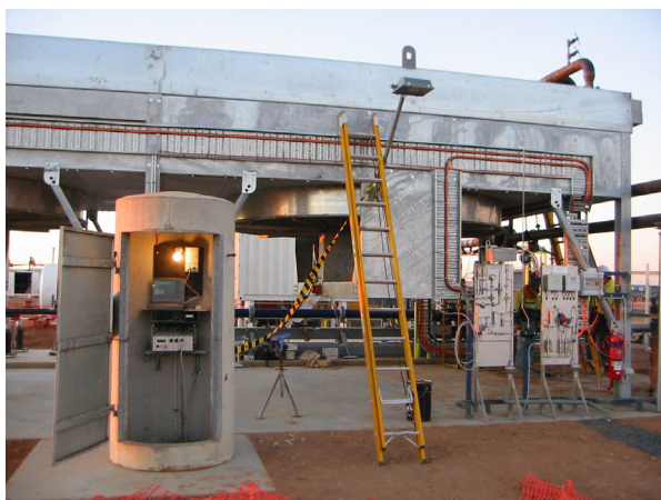
Figure 3: The fibre-optical fluorometer (left hand side) and fluid sampling panel (right hand side) used in the test carried out at the Habanero site.
