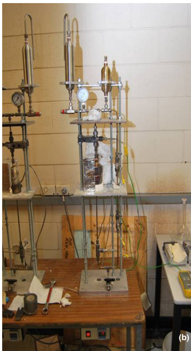
Figure 1: (a) Diagram of the flow through cell (b) Photograph of the geothermal flow through cell
