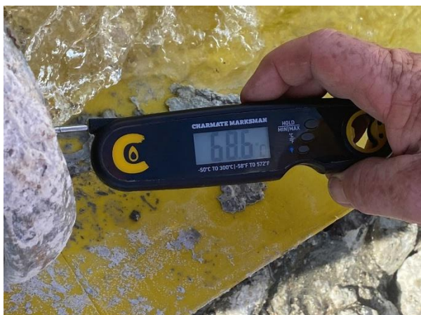
Figure 4: Temperature reading during early flow testing of the bore.
