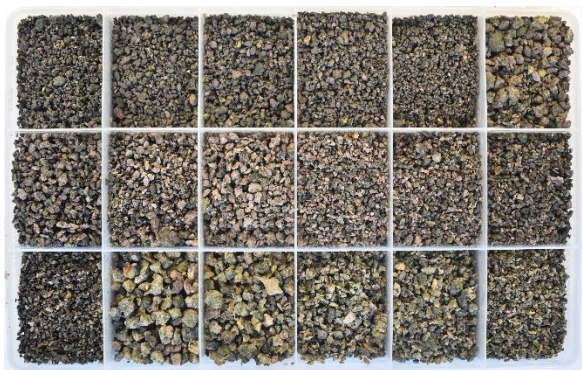
Figure 3: Example of archived chip samples (347–364 m) from BN23-0020
