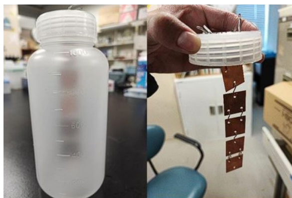
Figure 5: Suspended metal plates in a 1L polypropylene bottle for batch experiment of silica scale inhibition.
