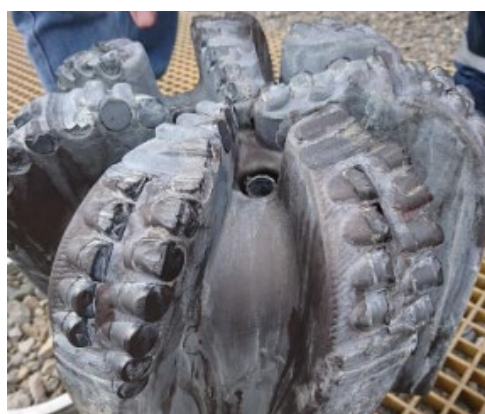
Figure 4. Old PDC Bit design run in NZ geothermal field
