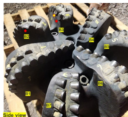
Figure 10. HD75DMF bit dull condition after run
