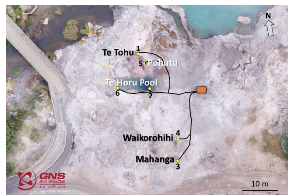
Figure 2: Aerial image of Geyser Flat, showing the layout of the temperature sensor network for Deployment 2. Yellow circles mark the sensor locations, black lines the connecting wires, and the orange rectangle the pelican case containing the datalogger and batteries.
