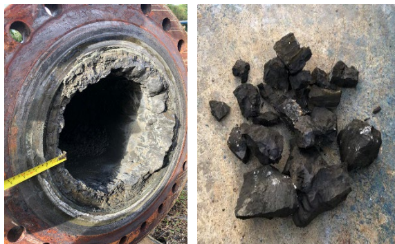
Figure 8: Scale in form of Iron Sulfide deposited in the production facilities.
