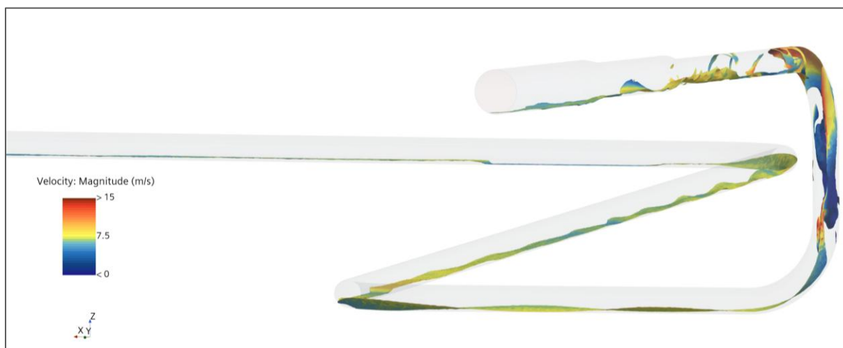
Figure 3: Final section of line leading into the separator showing the interface surface between gas phase and liquid phase, coloured by the velocity. Stratified flow leads into an unstable wavy-annular flow in the vertical riser.
